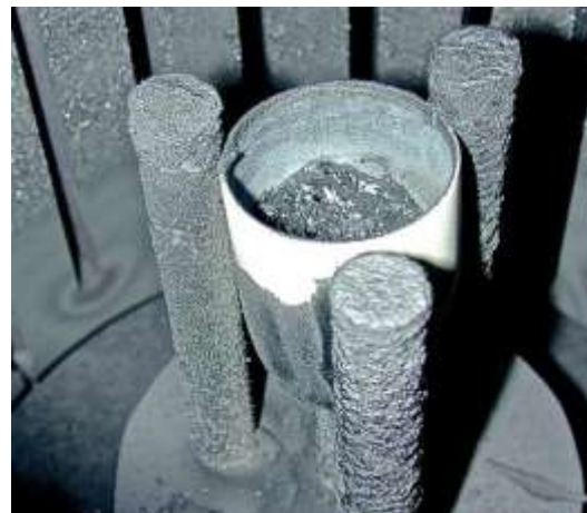
Figure 2. Deposits formed on rods and crucible during several melting runs.
