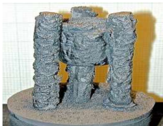
Figure 3. Rods and crucible entirely covered with silicon-colored deposit.
