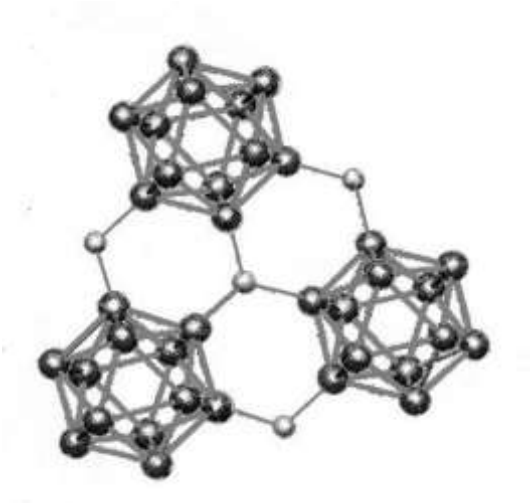
Figure 15. B_{12} -icosahedral network in the structure of B_6N as seen along the [111] -axis. The smaller circles stand for the N atoms.
